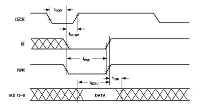
Figure 29. IDMA Write, Short Write Cycle
